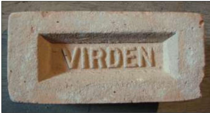
*Example of a machine-pressed brick manufactured at the Virden Brick & Tile Company, Manitoba between 1905 and 1915, with the company /community name impressed into the base of a deep frog. **VIRDEN** bricks are found in historic buildings throughout southern Saskatchewan.*
