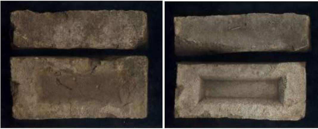
*Hand-mould bricks found at the Assiniboia Brick Yard site, with a shallow frog (left) and deep frog impressed into the brick.*
