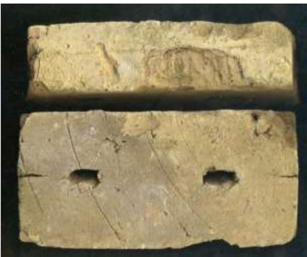
*An extruded brick, showing the curved striation marks confirm that the brick was wire cut. The rectangular holes reduce the brick weight and help hold the bricks to the mortar in a manner similar to the frogs in other types of bricks.*
